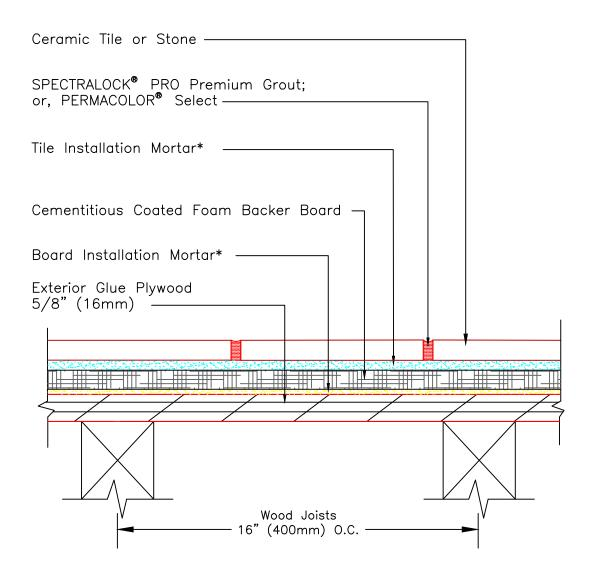
\* Board installation mortar and tile installation mortar to be either 254 Platinum, 257 TITANIUM™ or MULTIMAX™ LITE.
