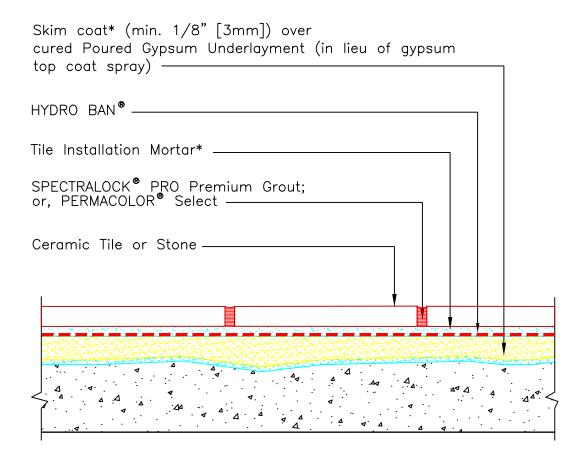
\* Skim Coat, and Tile Installation Mortar to be either 257 TITANIUM, 254 Platinum, or MULTIMAX LITE.
