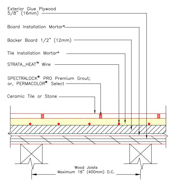
\* Board installation mortar and tile installation mortar to be either 254 Platinum, 257 TITANIUM™ or MULTIMAX™ LITE.
