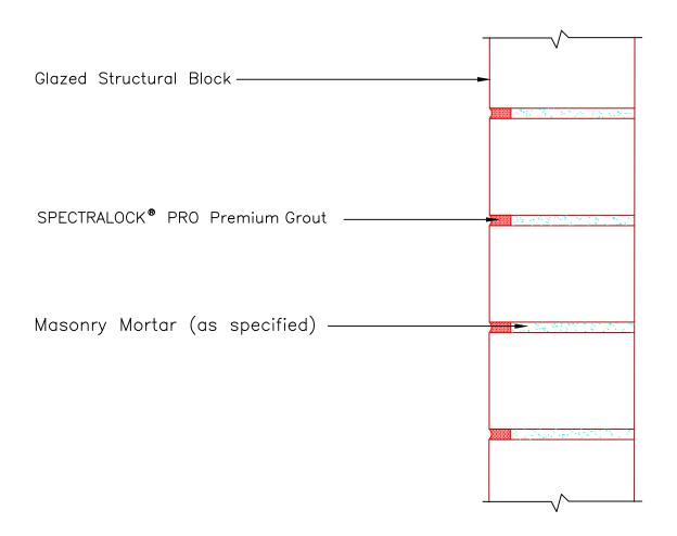
Structural Glazed Block with Joint Raked Back min. 3/8" (9mm).
