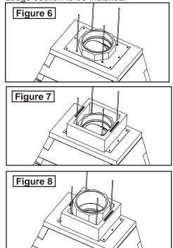
5. If an offset is required after a short run of straight flue, start with a standard 8" high inner flue (MCL-814). The offset will require that the inner and outer flue is flush at the beginning of the offset sections. After the offset is complete, resume the straight stack with a short 4" high inner flue (MCL-414) and continue with 8" high inner and outer sections (MCL-814, MCS-814). At the point
