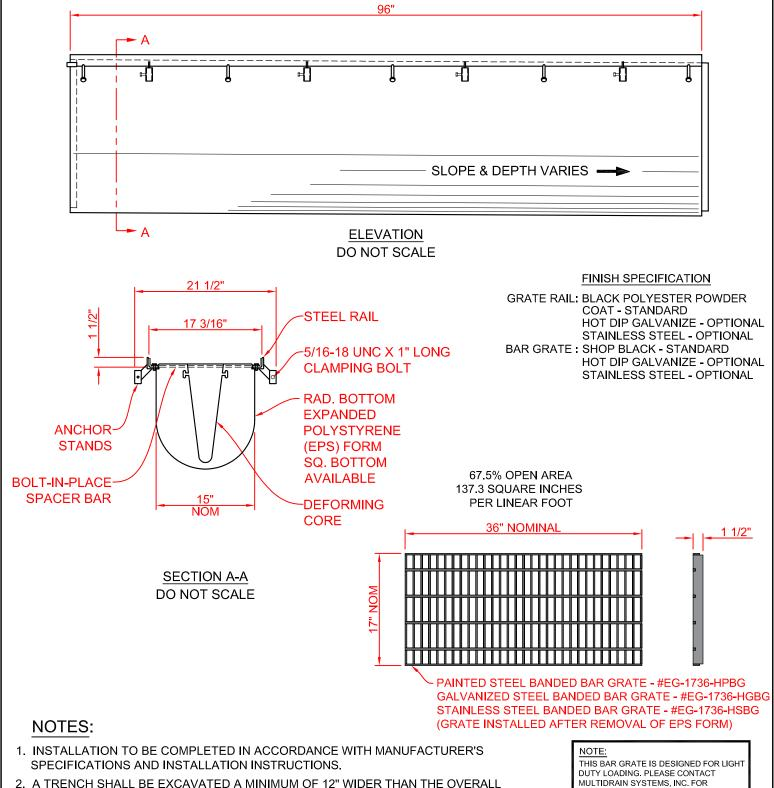
2. A TRENCH SHALL BE EXCAVATED A MINIMUM OF 12" WIDER THAN THE OVERALL WIDTH OF THE STEEL FRAME (6" MINIMUM ON EACH SIDE) AND A MINIMUM OF 6 INCHES DEEPER THAN THE OVERALL DEPTH OF THE ECONODRAIN EPS FORM.
