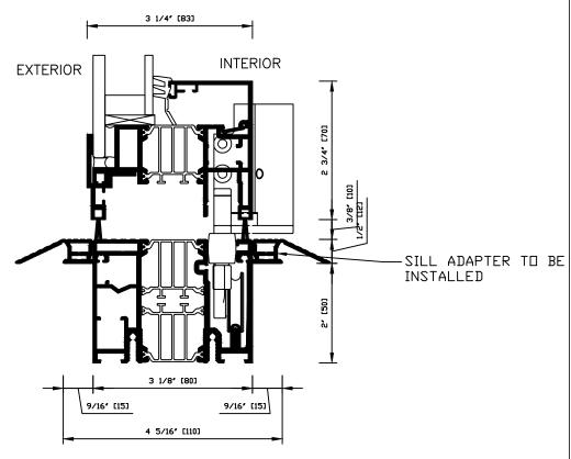
NOTE: SILL ADAPTER AND SCREWS PROVIDED BY NanaWall FIELD INSTALLATION BY OTHERS
