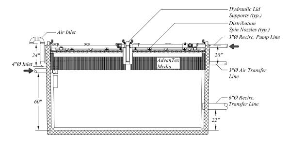
Spin Nozzles (typ.) AdvanTex Media 6"Ø Recirc.-Transfer Line Anti-floatation Assembly SECTION C-C
