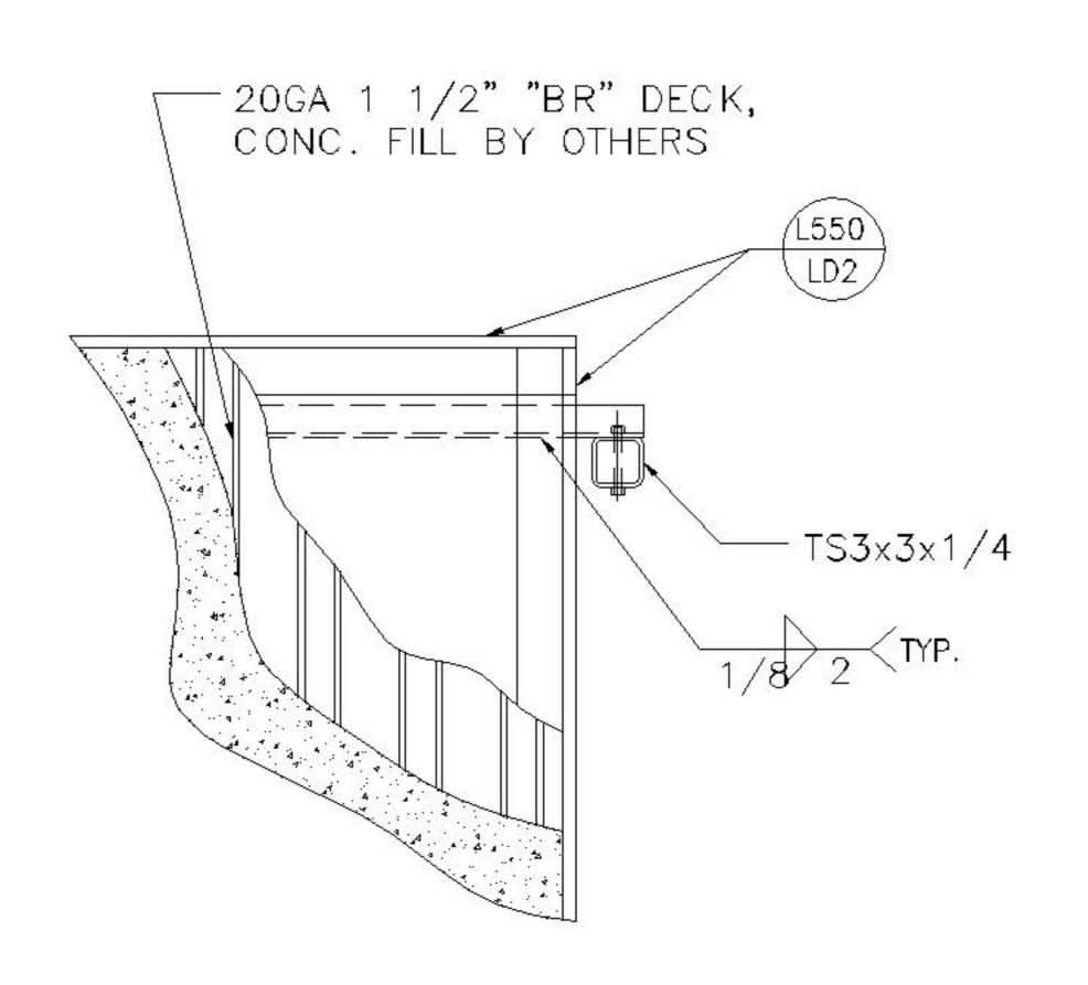
LANDING WITH "BR" DECKING TUBE STEEL LEG SUPPORT (CONCRETE FILL BY OTHERS)
