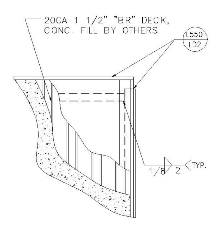
LANDING WITH "BR" DECKING LEDGER ANGLE SUPPORT (CONCRETE FILL BY OTHERS)
