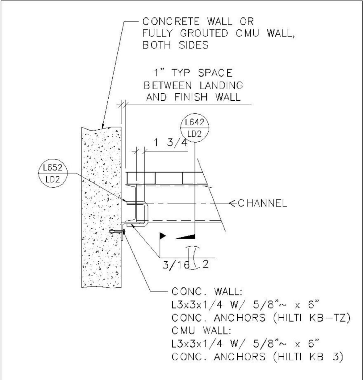
LANDING WITH FLOOR PLATE SEISMIC CONNECTION SUPPORT
