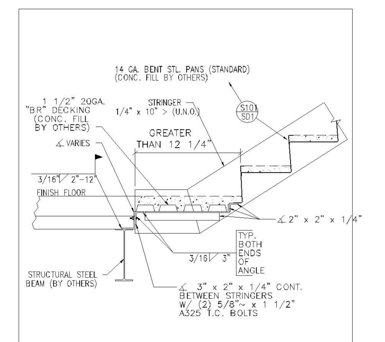
STAIR BOTTOM CONNECTION TO STRUCTURAL DECK EDGE W/ HAUNCHED TREAD (STANDARD)
