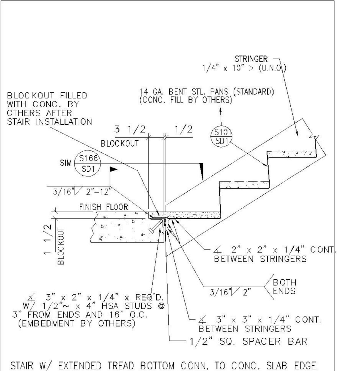
STAIR W/ EXTENDED TREAD BOTTOM CONN. TO CONC. SLAB EDGE (STANDARD)
