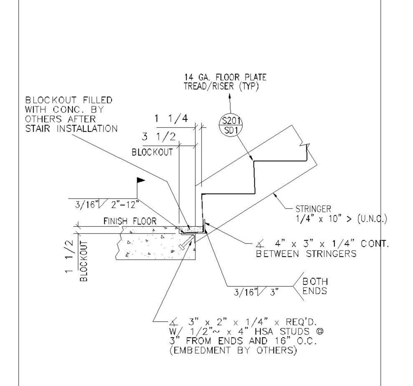
STAIR BOTTOM CONNECTION TO CONC, SLAB EDGE (STANDARD)
