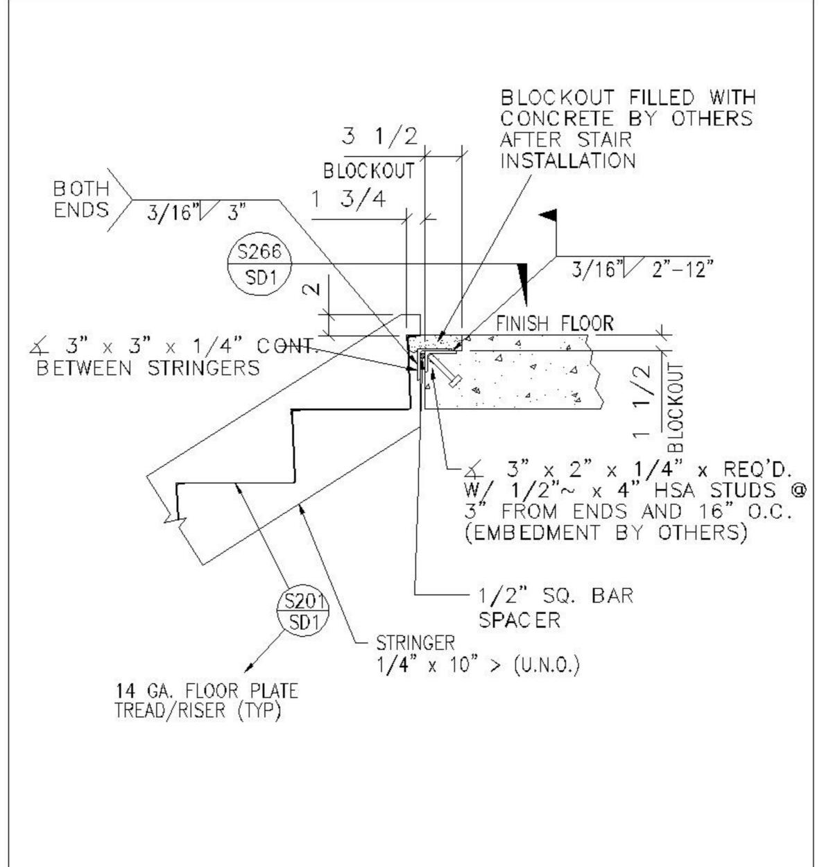
STAIR TOP CONNECTION TO CONC. SLAB EDGE (STANDARD)
