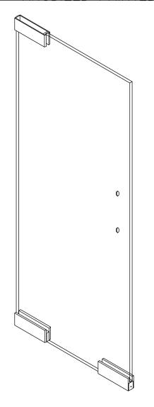
9½" PL-375 TOP PATCH (CLAD) BY P.R.L. GLASS 3/4" CLEAR TEMPERED GLASS-BY P.R.L. GLASS 9½" PL-375 BTM PATCH (CLAD) BY P.R.L. GLASS
