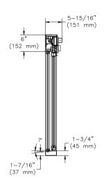
DUPLEX POWER CONNECTION POINT INSIDE OF HEADER BOTH SIDE FRAMES ARE HOLLOW FOR ELECTRICAL ACCESS FROM EACH CORNER LEADING TO THE HEADER. PRESENCE SENSOR
