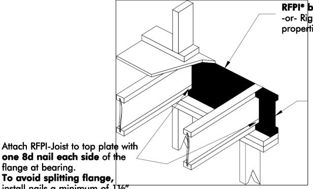
**RFPI** blocking panel vertical load transfer = 2000 plf maximum -or- RigidRim Rimboard (see Roseburg EWP Design Guide for design properties)
