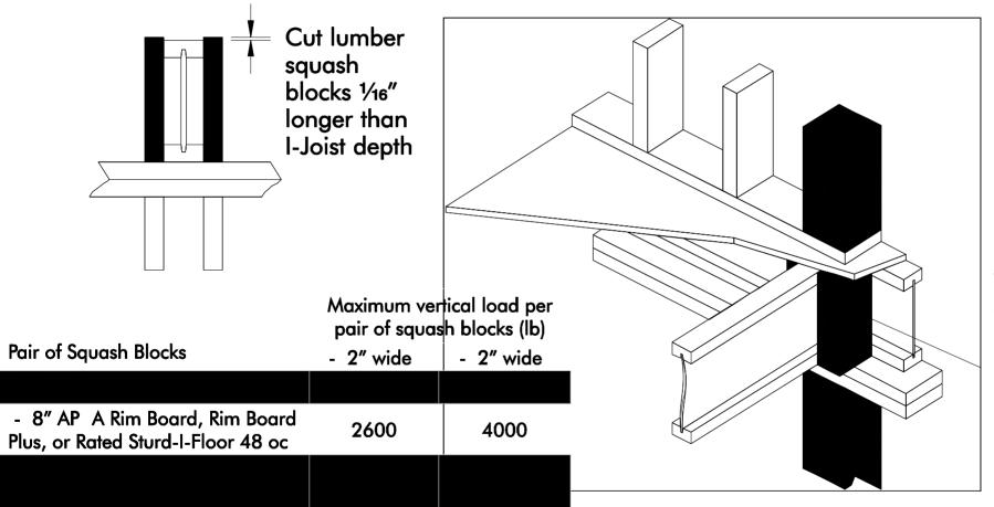
Solid Block all posts from above to bearing below. Match bearing area of blocks below to post above.
