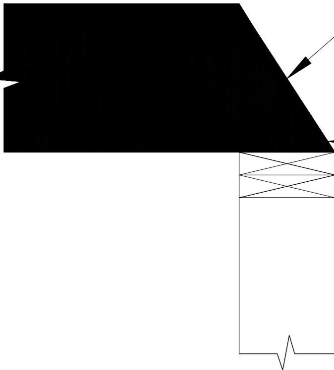
Do not bevel-cut joist beyond inside face of wall
