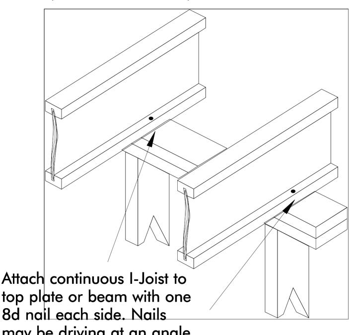
may be driving at an angle to avoid splitting of bearing plate.
