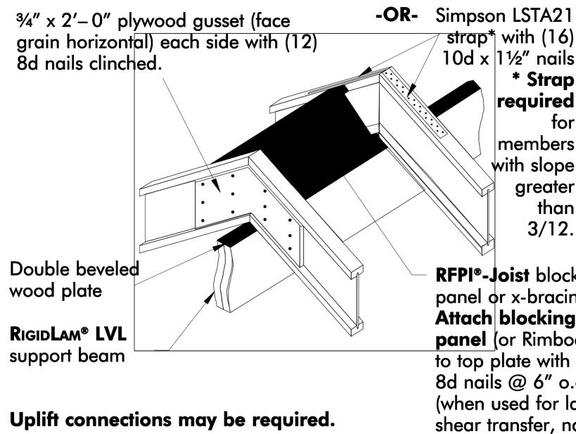
RFPI®-Joist blocking panel or x-bracing. Attach blocking panel (or Rimboard) to top plate with 8d nails @ 6" o.c. (when used for lateral shear transfer, nail to bearing plate with same nailing as required for decking)
