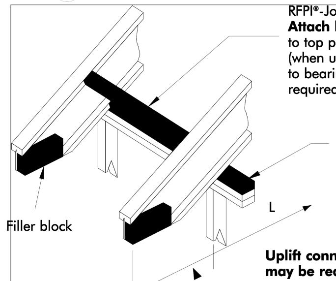
RFPI®-Joist blocking panel or x-bracing. Attach blocking panel (or Rimboard) to top plate with 8d nails @ 6" o.c. (when used for lateral shear transfer, nail to bearing plate with same nailing as required for decking)
