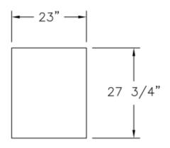
UNIT IS SHOWN WITHOUT A TOP, TOPS WOULD BE ST. ST. W/WOOD CORE, 29"D WITH OVERHANG IN THE FRONT & 1 5/32"H. CHECK CATALOG FOR PRE DETERMINED SIZES.
