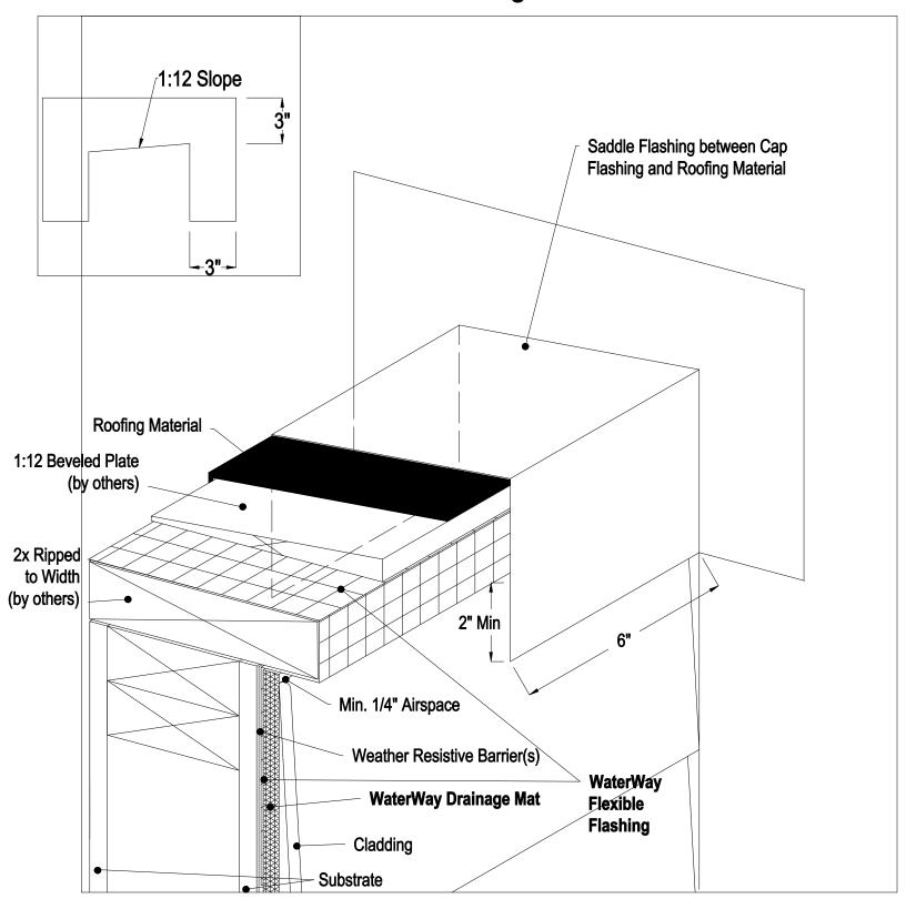
Note: Refer to Cap Flashing Detail (Flashing 3.01)
