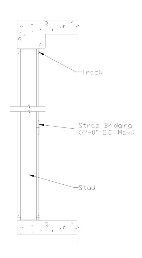
NOTE: BRIDGING TO BE INSTALLED PRIOR TO SHEATHING
