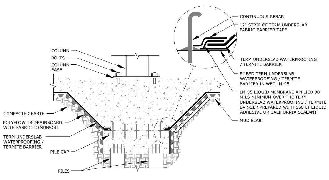
SECTION @ TERM® UNDERSLAB WATERPROOFING / TERMITE BARRIER GRADE BEAM PILE CAP (OPTION 2)
