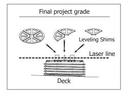
7. Adjust final pedestal height by using Uni-Shims™ whole or in segments at the top of pedestal assembly.
