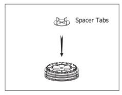
5. Complete assembly by snapping on Spacer Tabs in order to provide proper spacing of pavers. Spacer tabs are perforated and can be ripped or cut off.
