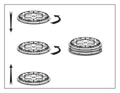
4. Assemble by rotating & aligning alphabets of one Stak-Cap™ with the Stak-Cap™ bellow it for slope compensation.
