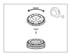
3. Using a laser determine final height of pedestals from ½" to 2-¼" high. Consider in calculation the Buffer Pads as 1/8" thick.
