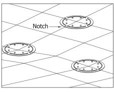
2. Position Buffer Pads on chalk grid lines using the v-notch as a reference point.
