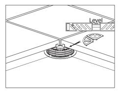
8. Use a spirit level to check level and use additional half or quarter Uni-Shims<sup>™</sup> for fine tuning of individual corners of pavers.
