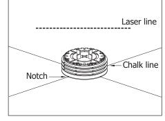
6. Position pedestal under laser line and align Buffer Pad notch with chalk line. Orient the pedestal assembly so that the top Stak-Cap $^{\text{TM}}$  pair high side points towards decline of slope.
