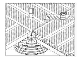
9. For IPE wood insert the lock washer in to the kurf-cut on the corners of wood tiles then insert screw through lock washer and hand tighten.
