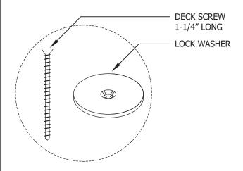
INSERT THE LOCK WASHER IN TO THE KURF CUT BETWEEN THE UPPER SLAT AND BOTTOM RAIL OF 3 WOOD PAVERS. INSERT THE 4th PAVER IN TO THE 4TH CORNER. ONCE ALL 4 PAVERS ARE TIGHTLY IN PLACE INSERT DECK SCREW (1-1/4" LONG) THROUGH LOCK WASHER AND HAND TIGHTEN IN TO PEDESTAL TOP UNTIL ALL 4 PAVERS ARE SECURELY FASTENED TO THE PEDESTAL. DO NOT OVER TIGHTEN.
