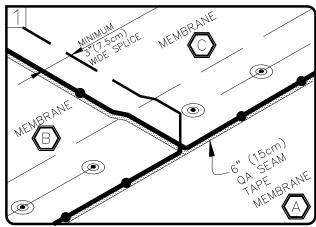
POSITION MEMBRANE TO ALLOW AN APPROXIMATE (17.5cm) OVERLAP ALONG THE LENGTH OF THE MEMBRANE & 4" (10cm) AT END LAPS. THE PRE-MARKED LINE ON THE MEMBRANE EDGE CAN BE USED AS A GUIDE FOR TAPE PLACEMENT.
