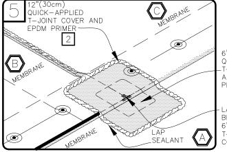
APPLY 6"(15cm) QUICK-APPLIED T-JOINT COVER AND 12"(30cm) QUICK-APPLIED T-JOINT COVER OR QUICK-APPLIED UNCURED EPDM CENTERED OVER THE INTERSECTING POINT OF THE LEADING EDGES OF THE FIELD SPLICE INTERSECTION AS SHOWN.
