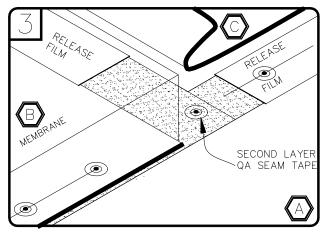
SPLICE SHEET B TO SHEET A AND APPLY SECOND PIECE OF QA SEAM TAPE BETWEEN SHEET B AND C. RELEASE FILM AS SHOWN.
