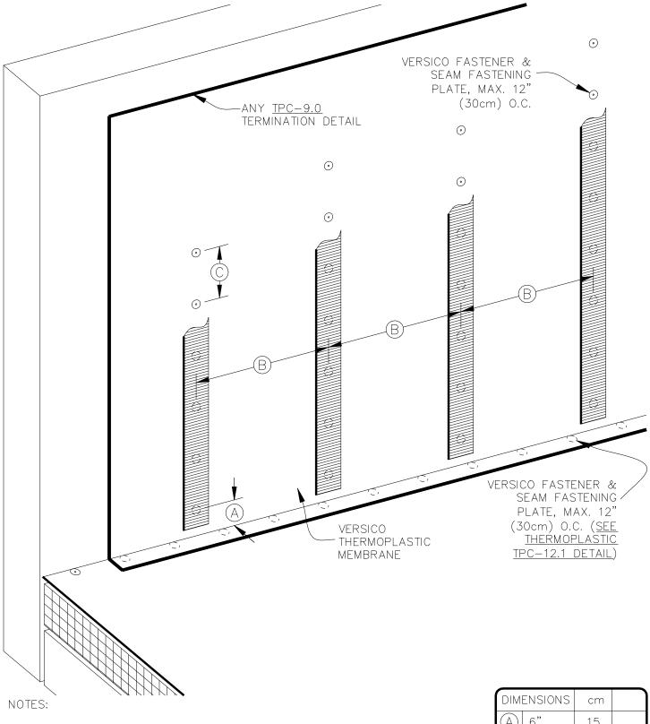
1. FOR TPO, USE 6" (15cm) WIDE PS COVERSTRIP, FOR PVC USE 6" (15cm) WIDE REINFORCED PVC MEMBRANE, HOT AIR WELD ALL EDGES WITH MIN. 1-1/2" (4cm) PAST FASTENING PLATES
