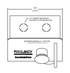
NOTE: INSTALL ALL CONSOLE PORTS WITH E-STOPAT SWITCH HEIGHT, 44" FROM FINISHED FLOOR, ALL CONSOLE PORT AND REMOTE E-STOP LOCATIONS ARE TO BE CONFIRMED WITH THE END USERS' SITE CONSULTANT AND J.R. CLANCY CONTROLS DEPARTMENT BEFORE MOUNTING.
