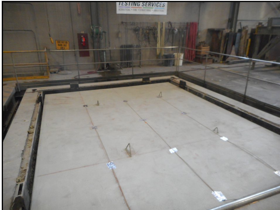
Unexposed Side – Pre-Test (Prior to Loading Tank Placement)
