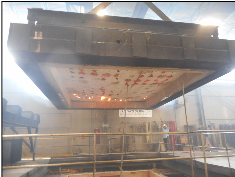
Exposed Side – Post-Test (Removing from Furnace)
