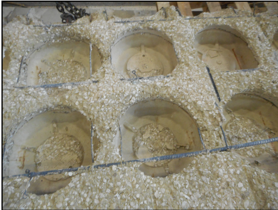
Exposed Side – Post-Test (Close-up of Plastic Void Locations)
