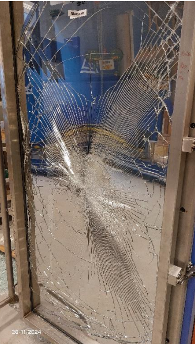
Picture 4. Sample 4 After impact
