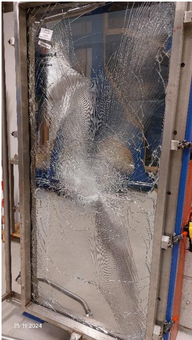
Picture 4. Sample 4 After impact
