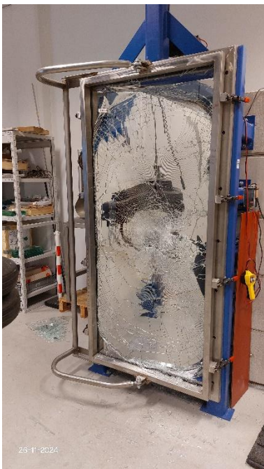
Picture 3. Sample 3 After impact
