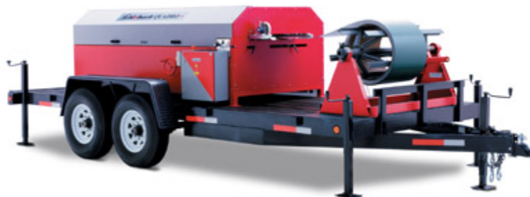
Figure 2: Mobile Roll Former (Photo courtesy Schleich Machines)
