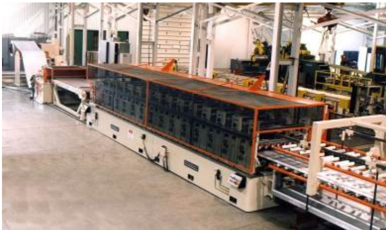
Figure 1: Inline Roll Former (Photo courtesy The Bradbury Co.)
