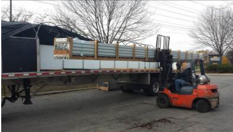
Figure 4: Metal roof and wall systems are generally transported by truck from the factory to a job site as shown in this picture. They can also be loaded into closed containers for transport by rail or ship.
