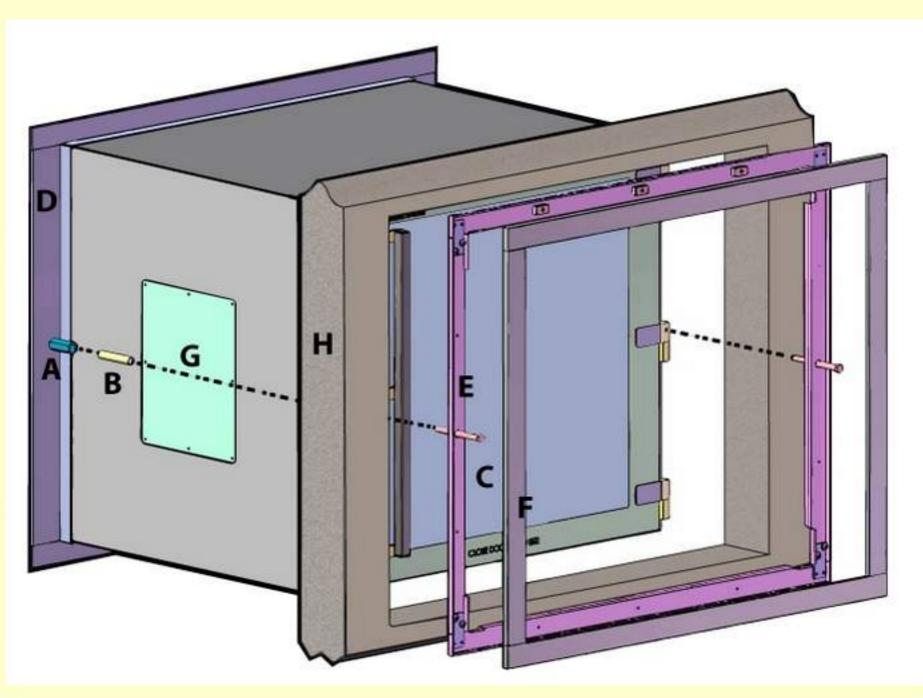
Unique quick-mount system allows installaion in a finished wall cut-out
