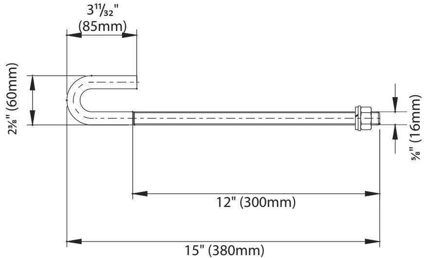
USE: Threaded anchor bolt for self-supporting carriages.
