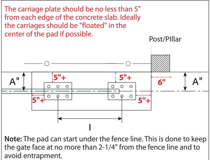
**Note:** The top of the bolt/tie rod should stick out of the cement at least 2". Keep nut on top of concrete, do not sink in.
