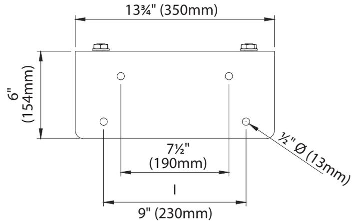
USE: Guide plate for sliding gates and self-supporting.
