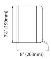
TYPE: Lower striker for fixing. FIXING: For fixing on post or for fixing on special bracket CG-15.
