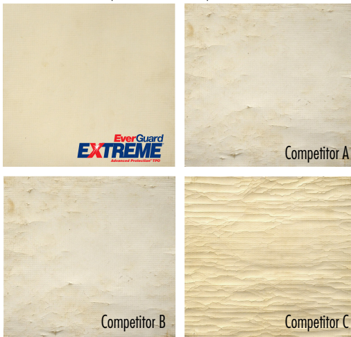
Images represent how samples look compared to EverGuard Extreme ® TPO after heat aging for 8 hours a day at 275°F (135°C) for 161 days.
