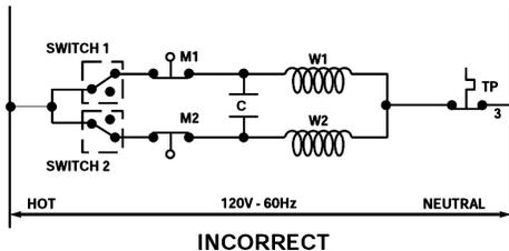
Because of the type of motor (asynchronous with built-in capacitor) and the built-in limit switches, it is crucial to follow two important recommendations to assure proper operation of the motorized systems. (Somfy® operators are not universal motors.)
