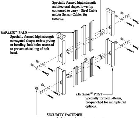
Stainless steel security nut prevents tampering or removal by normal tools.
