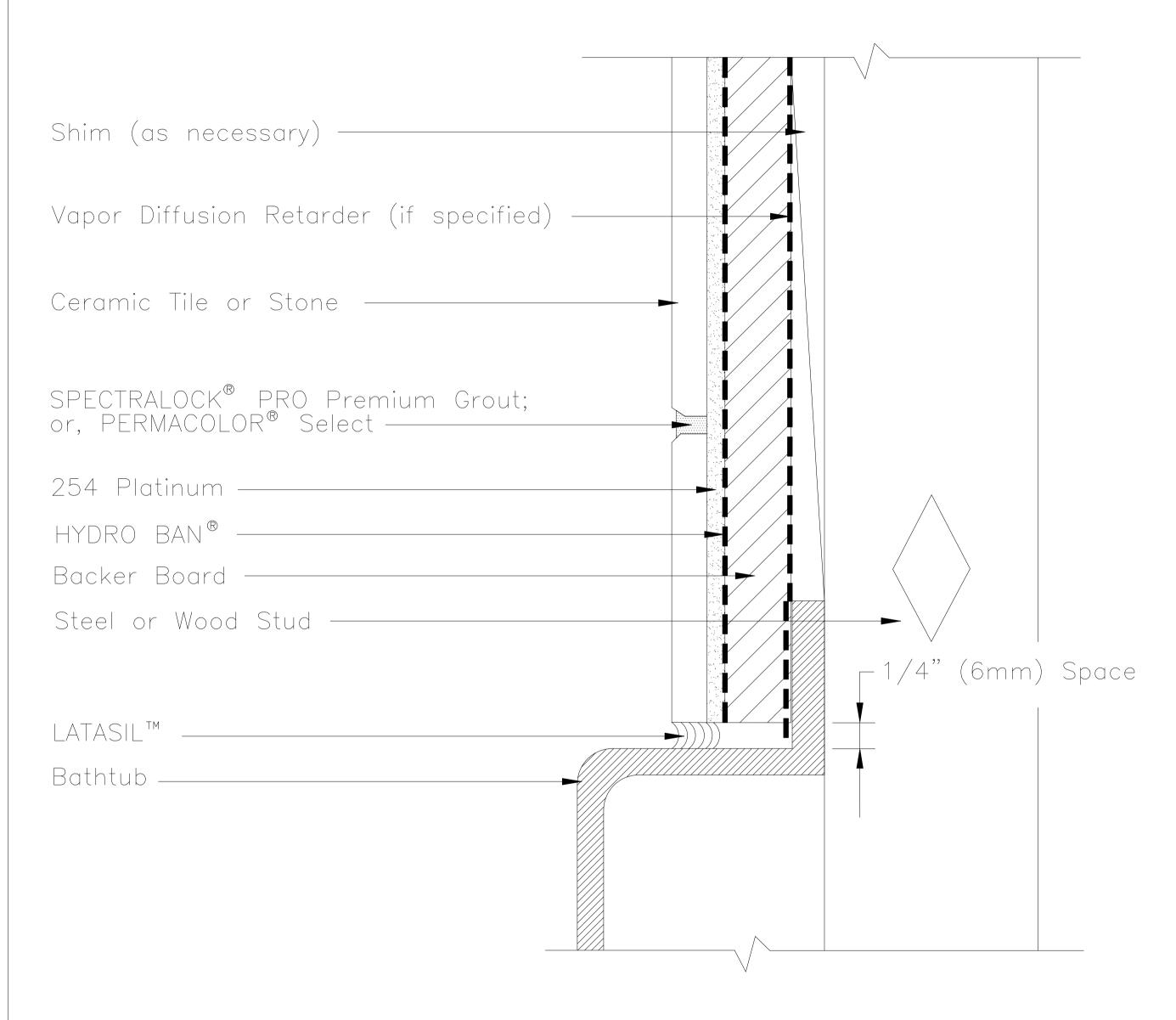
NOTE: Vapor diffusion retarder use, type and location to be determined by project design professional. May require leaving weeps open in sealant.
