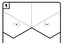
FASTEN MEMBRANE AND FLASH CURB OR WALL WITH CURED EPDM MEMBRANE FOLLOWING STANDARD PROCEDURES USING BONDING ADHESIVE AND QA SEAM TAPE AT MEMBRANE SPLICE.
