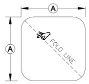
CUT A SECTION OF THERMOPLASTIC NON-REINFORCED MEMBRANE WITH ROUNDED CORNERS
