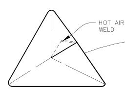
POSITION AND HEAT WELD CORNER IN PLACE AS SHOWN
